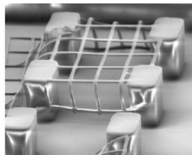
Figure 7. Suspended 10 \mu\text{m} thick grid structures on the top of 100 \mu\text{m} height SU-8 pillars made by gray scale lithography. (Reprinted from ref 78, Copyright 2003, with permission from Elsevier.)
